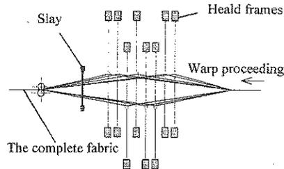
Figure 1. Drafted process of weaving
